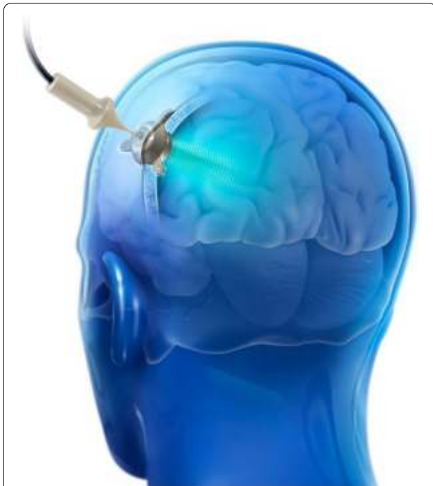
Fig. 1 The SonoCloud-1 is a 1-MHz implantable ultrasound device that is implanted within the skull thickness (extradural) and activated at each treatment cycle by connecting it using a transdermal needle to an external radiofrequency generator. In this study, the SonoCloud-1 was implanted to target and temporarily disrupt the BBB above the left supramarginal gyrus
